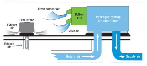
A bolt-on ERV system attaches to your existing air-conditioning unit. It draws its exhaust air only from the return duct. An exhaust fan is still required for spaces such as offices, restrooms and breakrooms.
