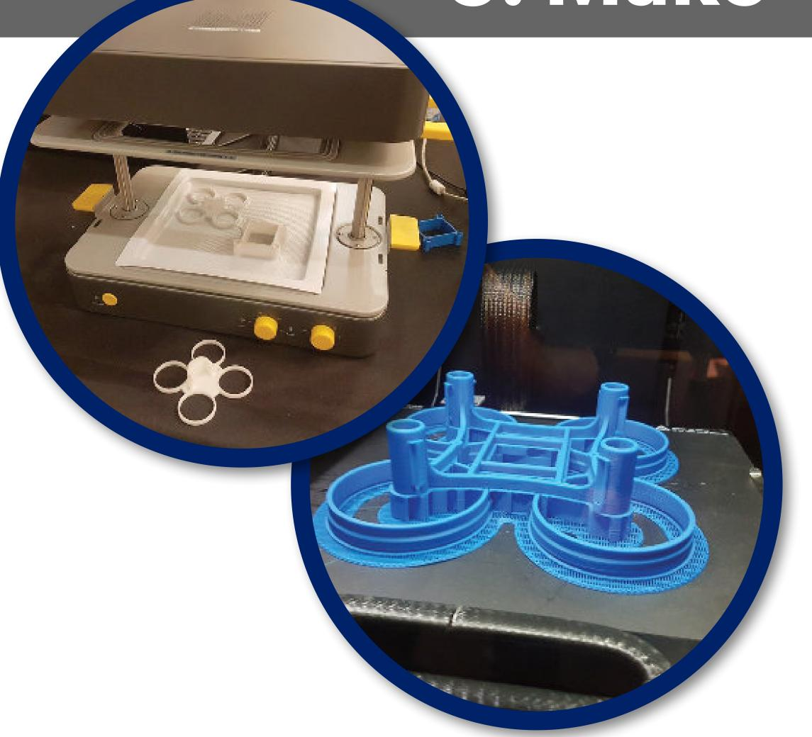
Students manufacture and assemble a racing drone using modern rapid prototyping technology. During the manufacturing process students complete and document multiple iterations until a successful prototype is ready for testing.
